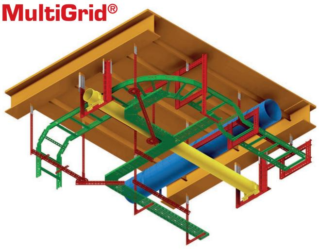
In order to provide ultimate flexibility during installation and future extension or adaptation, we highly recommended designing and installing according to our MultiGrid® concept for support.
